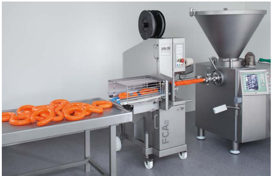
FCA 80 with adjusted front flap and double-conveyor belt specifically for rings
